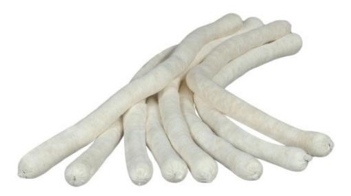
Oil Only absorbents are designed to be used around water sources to soak up oil while repelling water. These "medium" socks are sold 40 to a case, measure 3" in diameter and 4' in length and, are used to surround a spill to prevent it from spreading and causing further damage.
